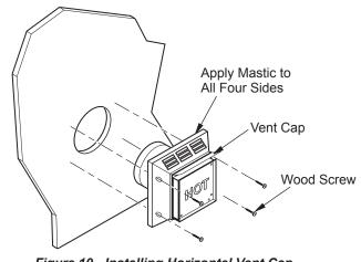
Figure 10 - Installing Horizontal Vent Cap (Noncombustible Exterior)
